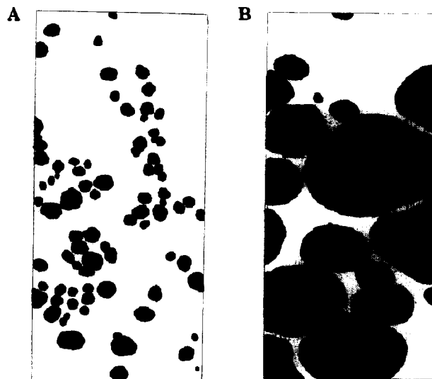
Figure 1. Typical image micrographs of oil in water emulsions stabilized by 0.3% native BSA obtained with a computerized diode array imaging system to magnify light microscope image at oil volume fractions of (A) \phi = 0.22 and (B) \phi = 0.62 . Original magnification = 2940 in x direction and 4900 in y direction. The micrographs have been reduced to 30% of their original magnification.
